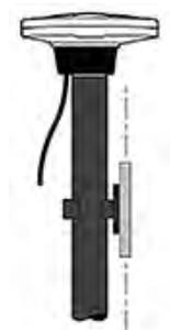
**IMPORTANT:** Your device must be attached parallel to the pole, so that the camera is pointing horizontally with respect to the Catalyst DA2 receiver.
