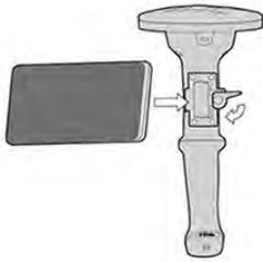
Make sure your device's USB C socket is on your left when the device is mounted on the SiteVision system.
