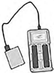
The battery charger will charge two batteries simultaneously and provides information on the level of charge. Depending on the level of battery charge, charging the batteries fully may take over 6 hours.
